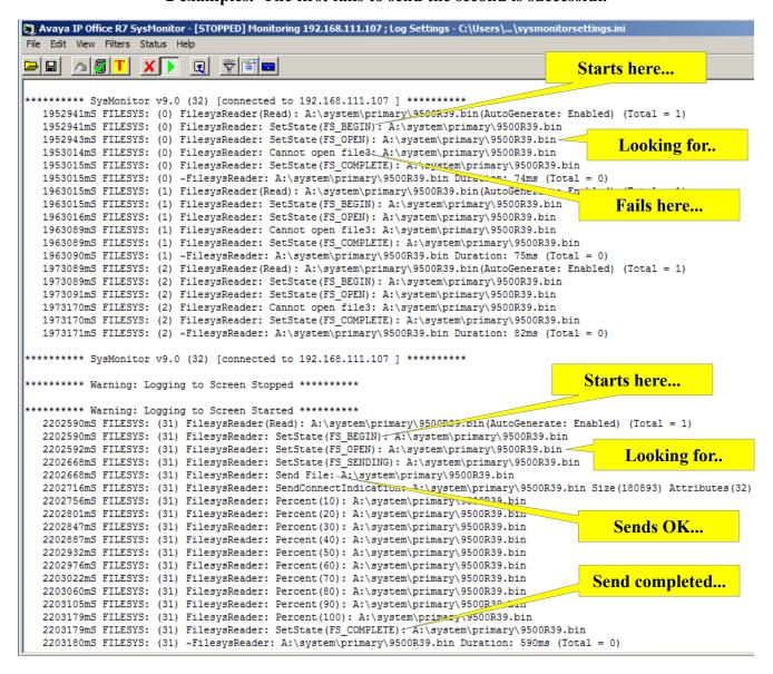
Configure the Monitor as shown on Page 1. Then when it is running, plug in the phone to be tested. Watch the screen of the Monitor.
